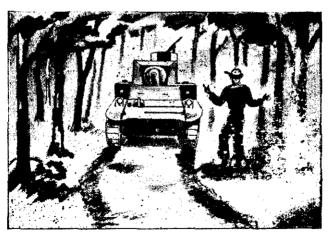
When backing into concealment, dismount and assist the driver by signaling the direction.
